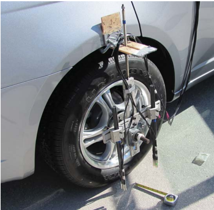
Left: North Carolina Agricultural and Technical State University (NCAT) OBSI test system. Right: Illingworth & Rodkin, Inc., OBSI test system.
