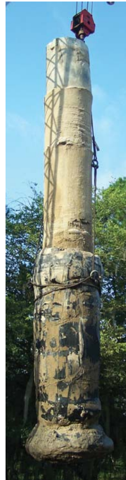
Left: The anatomy of a jet-grouted pile. Right: An excavated test jet-grouted pile exhibits full bottom and side grout coverage. Due to the side grouting, the tip grout will not flow upward, but is forced to flow both sideways and downward, forming a bulb under the pile and increasing resistance.
