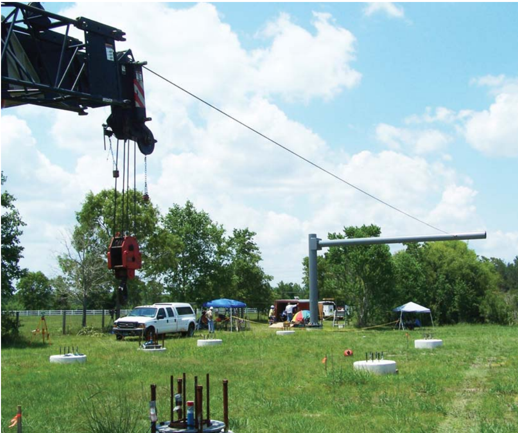
Left: Engineers conduct the torsional load tests using a full-scale FDOT mast arm assembly. The pole was mounted on a footing fixed to the top of a jet-grouted pile. During the test, researchers applied incremental horizontal loads to the mast arm using the cable of a winch attached to the tip of a crane boom.
