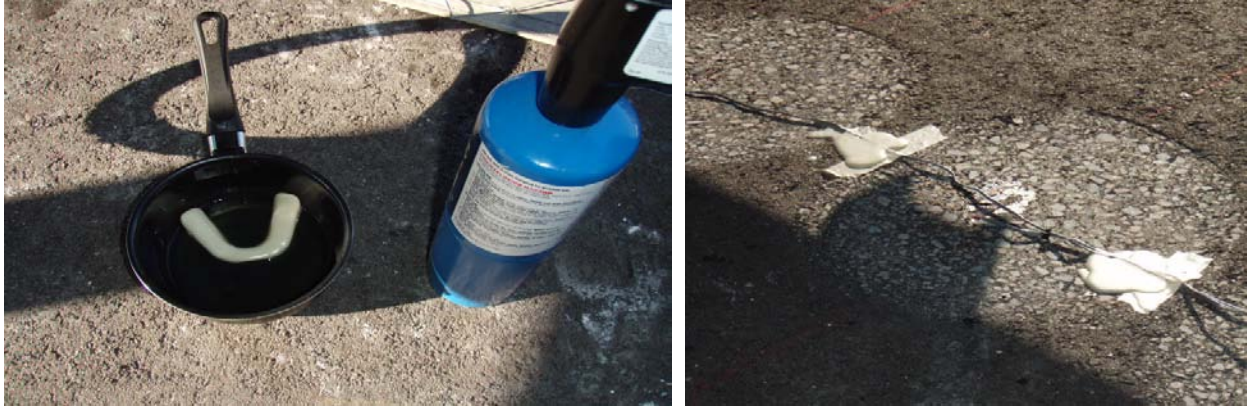
FIGURE 12 Melting wax and securing gauge wire.
