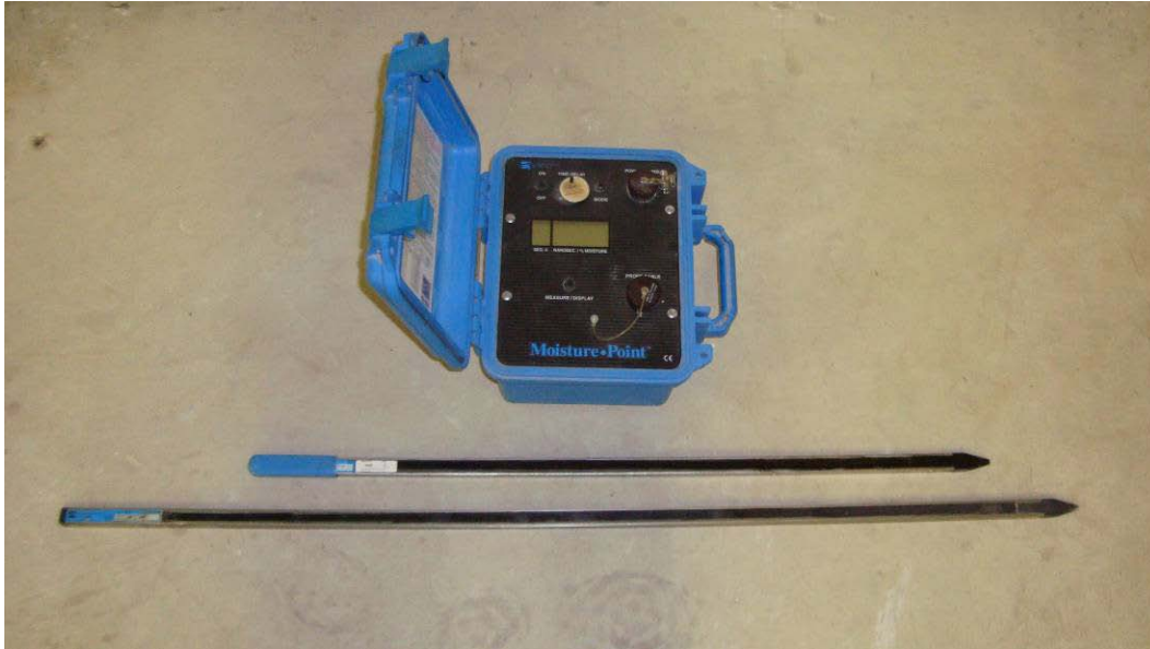
FIGURE 24 Moisture probes and data logger.
