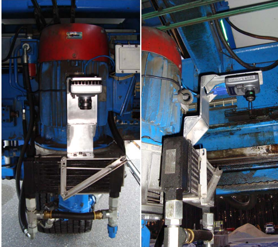
FIGURE 21 Camera mounted for crack detection.
