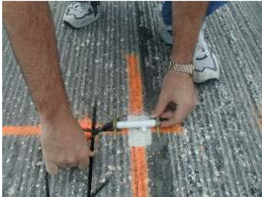
FIGURE 5 Placement of strain gauge and wires.
