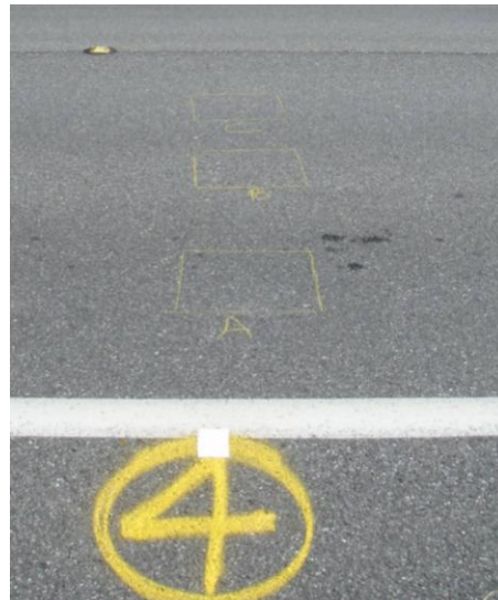
Figure 4. Schematic of coring operation for each location
