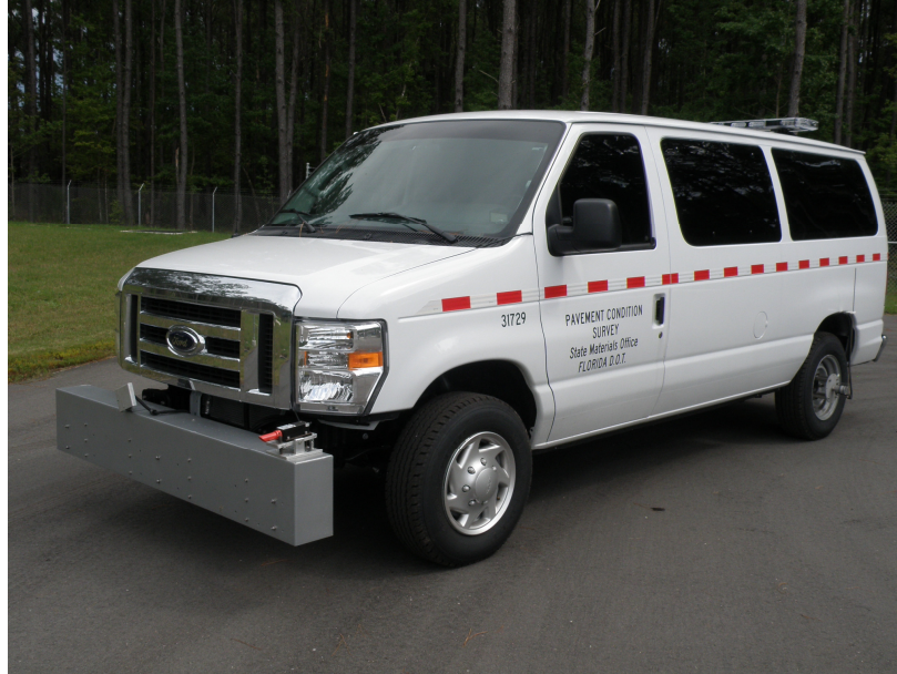
Figure 1. FDOT High-Speed Inertial Profiler
