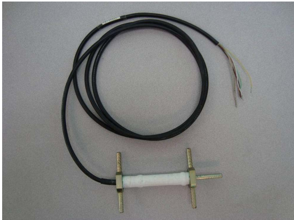
FIGURE 13 Asphalt strain gauge.
