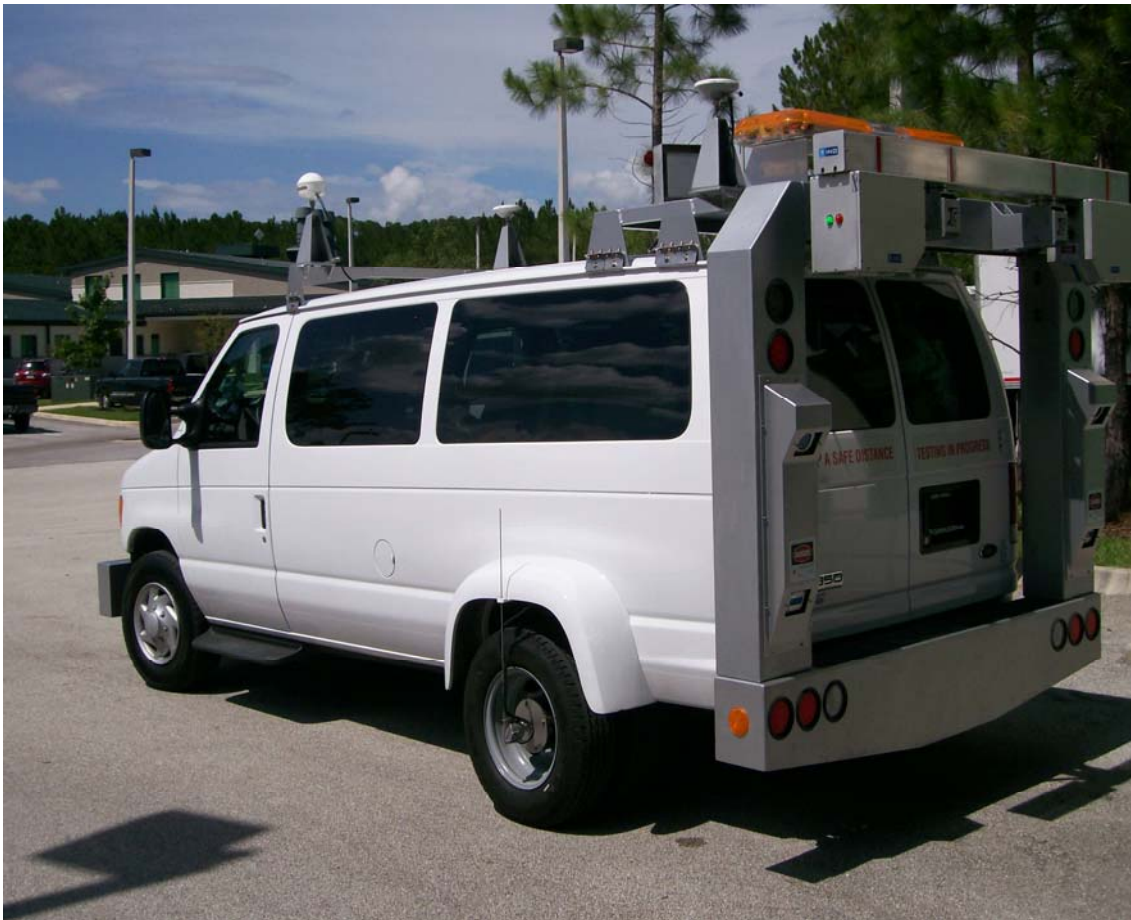
Figure 3. High-Speed Inertial Profiler (HSIP)
