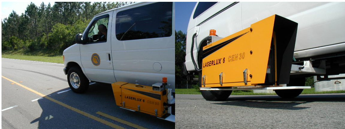
Figure 1. A Photographic Illustration of a Mobile Retroreflectometer Unit.
