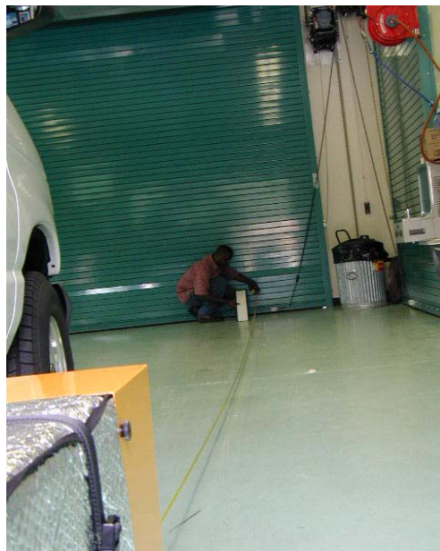
Figure 6. Placement of Striping Standard for MRU Calibration
