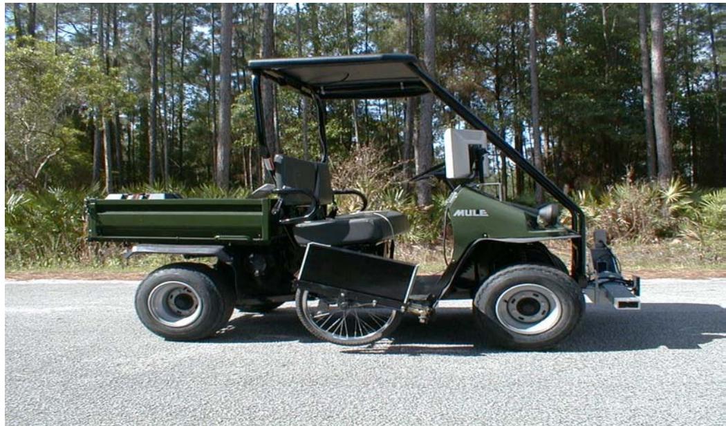
Figure 2 Illustration of a Lightweight Profiler.
