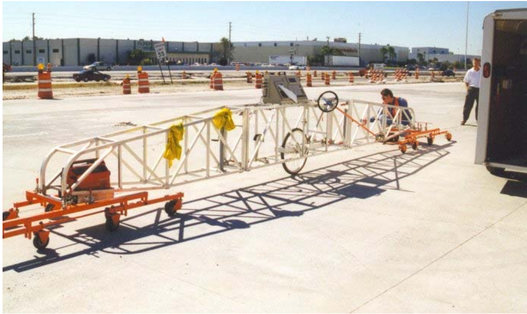
Figure 1 Illustration of a California-Type Profilograph.
