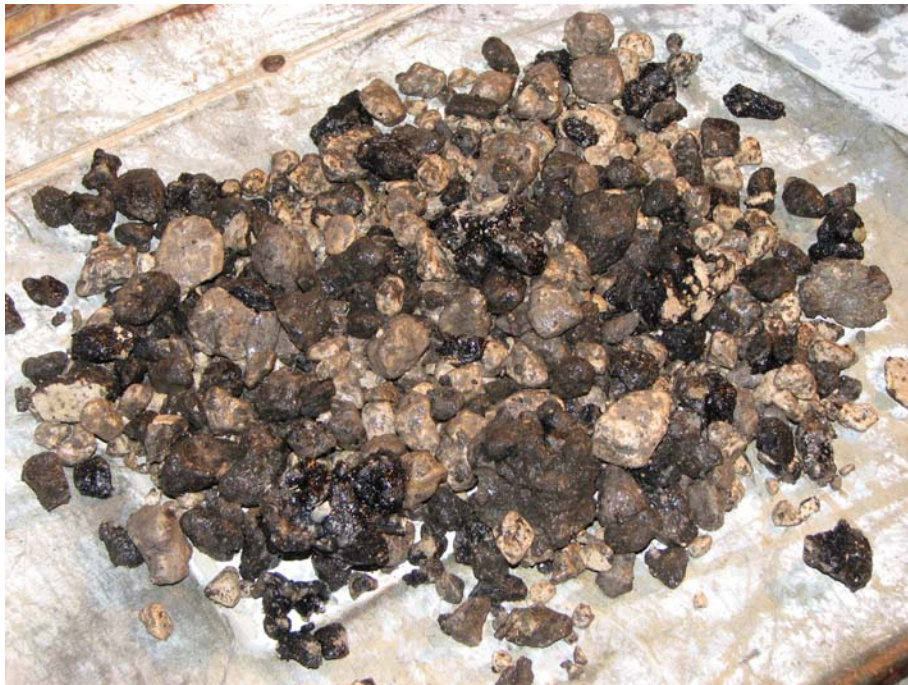
Figure 8 – Uncoated Aggregate from ATPB Layer; SR-60 and North 22nd Street - Hillsborough County
