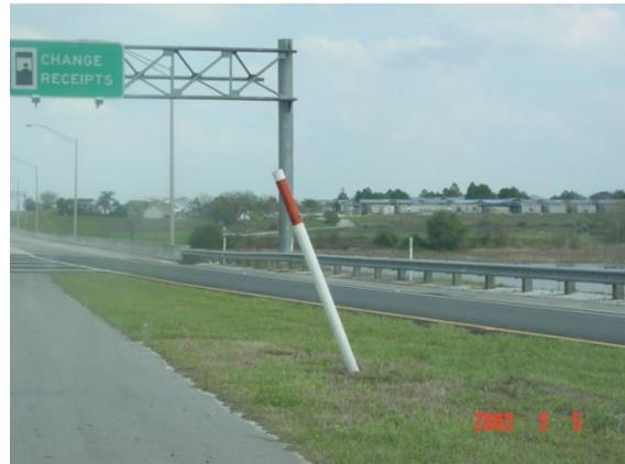
This object marker is for fiber optic cable. It would not be rated since this is not a Department maintained object.
