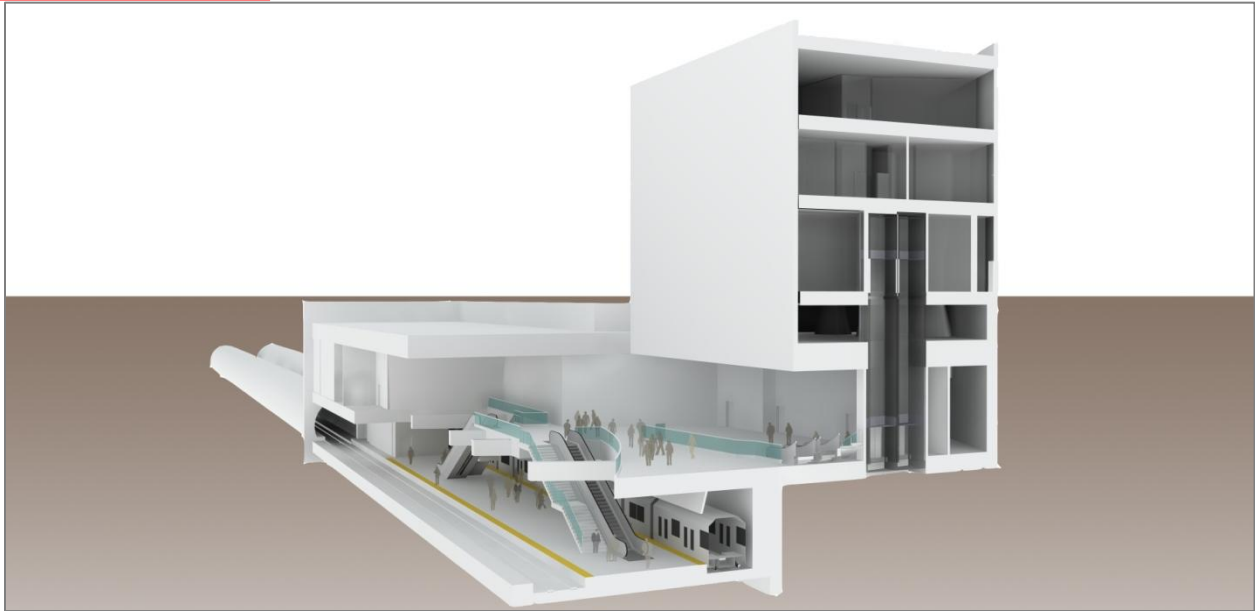
Figure 2-13: Two-Level Underground Station Sections
