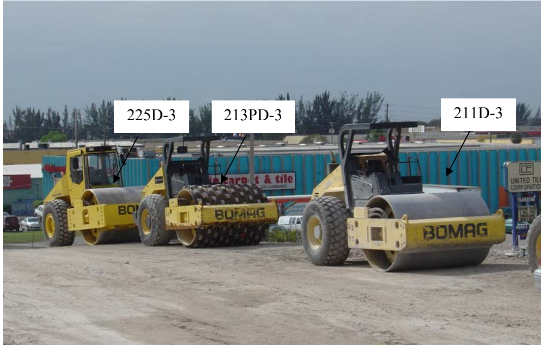
Figure 3.3 Test Section Compactors
