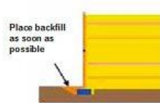
Figure 55, Place Backfill in Front of the Wall as Soon as Practical
