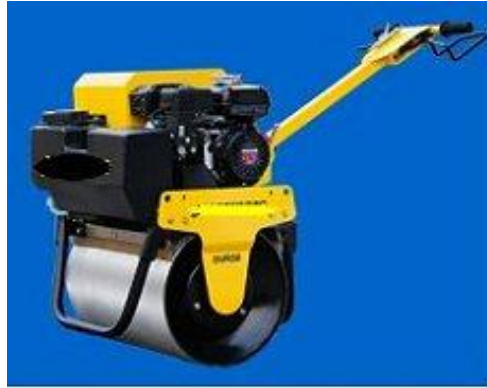
Figure 53, Typical compaction equipment used within 3 feet from the panel (must weigh less than 1000 lbs)
