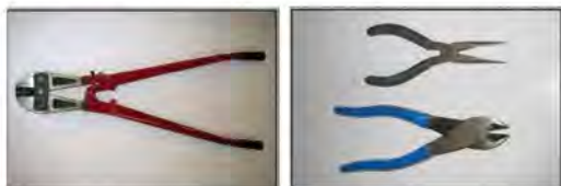
Figure 14 - Unsafe Cutting Tools
