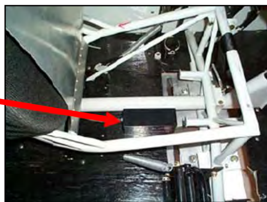
Figure 4: Electronic Module Assembly (EMA) Location
