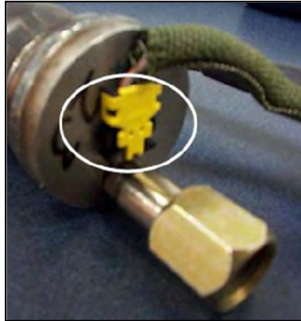
Figure 5: Connector attached to the Inflator Assembly
