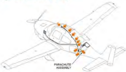
Figure 7 - Cable Routing: Handle to Rocket
