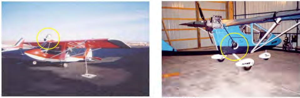
Figure 2 - Externally Mounted BPS
