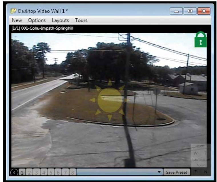
*Translucent controls that allow the operator to PTZ, go to/save preset location, and alter the focus of the camera.*
