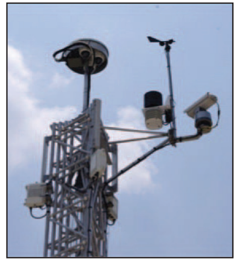
The camera housing is adjacent to the weather station on the trailer tower-top.
