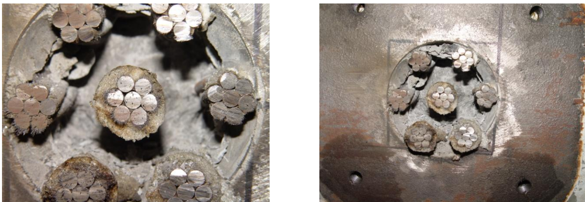
Figure 46. 7-strand - Second Specimen - Tendon Slip at Free face
