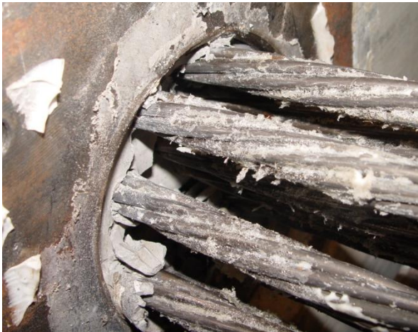
Figure 100. 12-strand - Third Specimen - Free Face – Post-active Loading Photo
