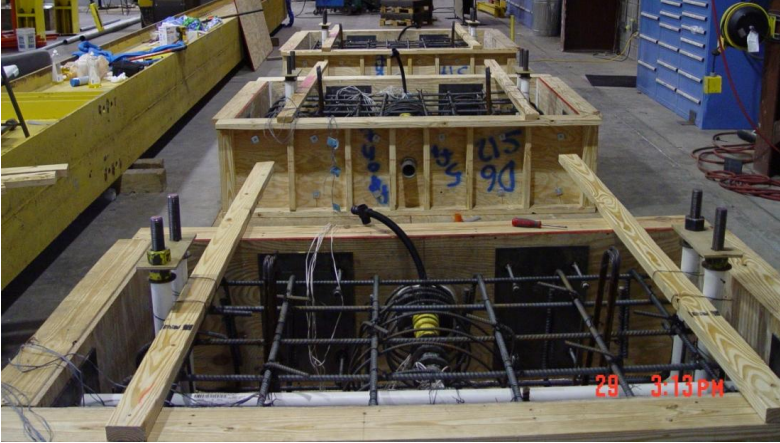
(a) Specimen Formwork Before Casting
