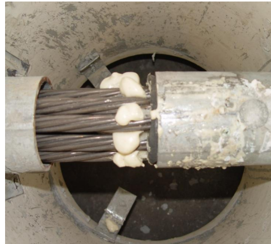
Figure 85. 12-strand – Second Specimen – Post-active Loading - Active Loading End Photo
