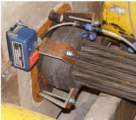
Figure 101. Free-end Grout Block Wedge Plate
