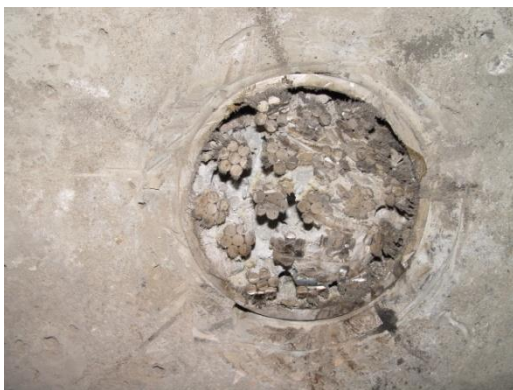
Figure 139. Second 19-strand Specimen Photo- Destressing End - After Pullout
