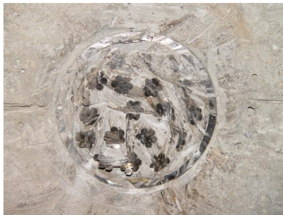
Figure 153. Third 19-strand Specimen Photo - Destressing End- After Active Loading
