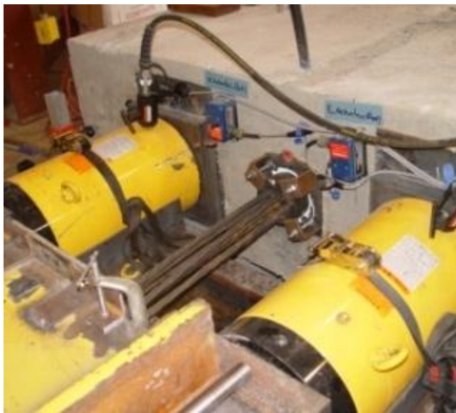
(b) Stressing Jacks
