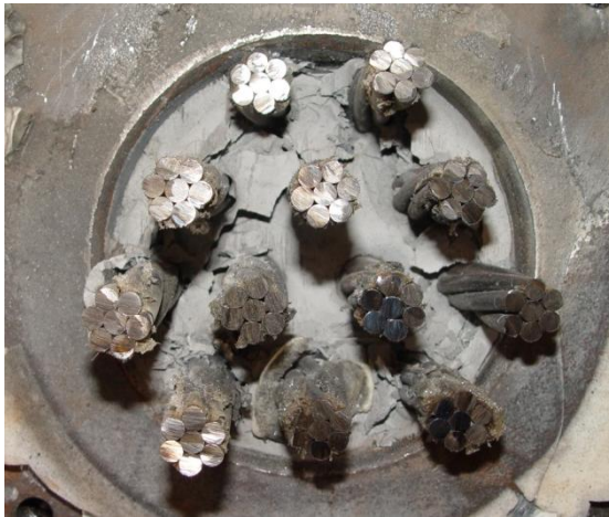
Figure 100. 12-strand - Third Specimen - Free Face – Post-active Loading Photo
