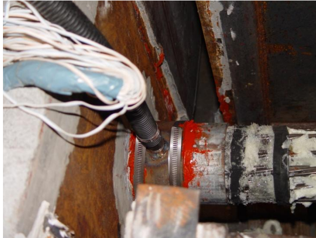
Figure 138. Second 19-strand Specimen Photo- Active Loading End After Pullout
