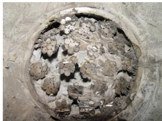
Figure 139. Second 19-strand Specimen Photo- Destressing End - After Pullout
