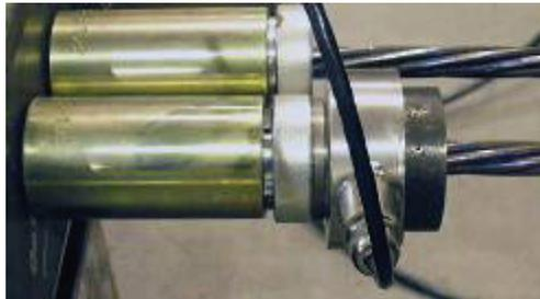
Figure 17. Load cell to verify applied pressure
