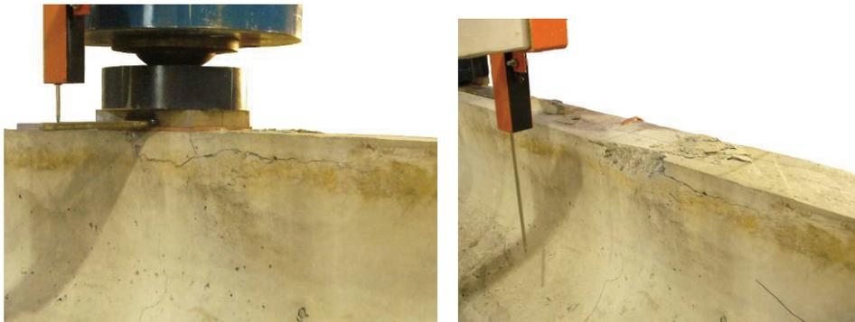
Figure 23. Failure of the compression zone for ITS
