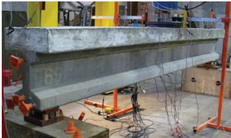
Figure 47. Pretensioned girders test setup.
