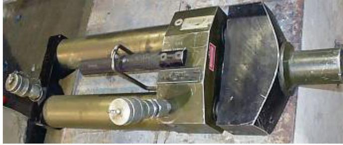
Figure 16. Monostrand jack used to post-tension ITO
