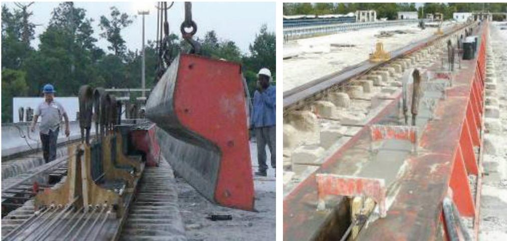
Figure 15. Prestressing strand and reinforcement cage during form placement. Casting bed for inverted tees
