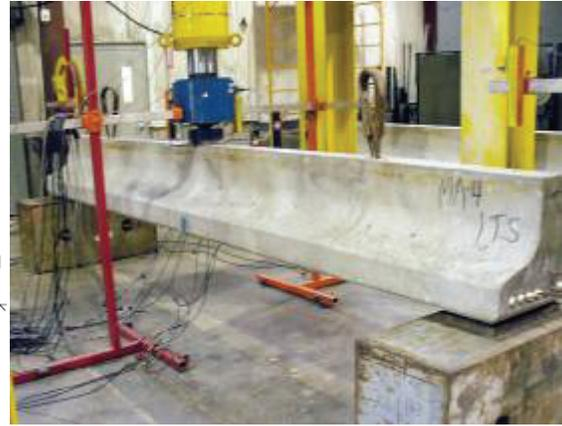
Figure 19. Test setup for inverted tee test.
