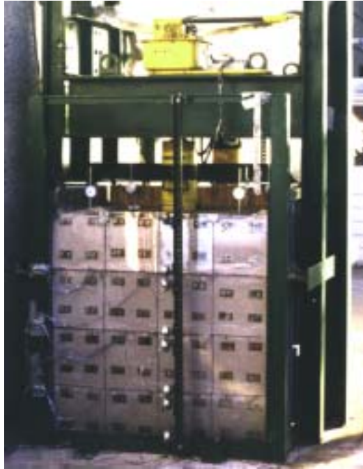
Figure 6.11. Finished small-scale MSE wall for HDPE geogrids
