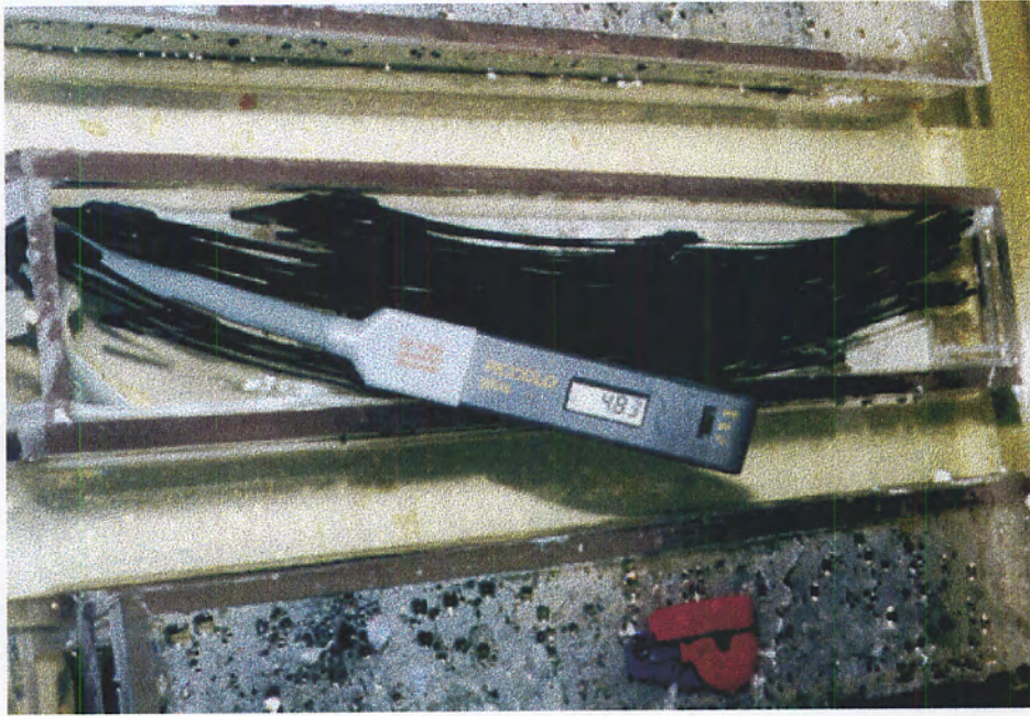
Figure 8.8 pH control, Phosphate (pH = 4.5) tank
