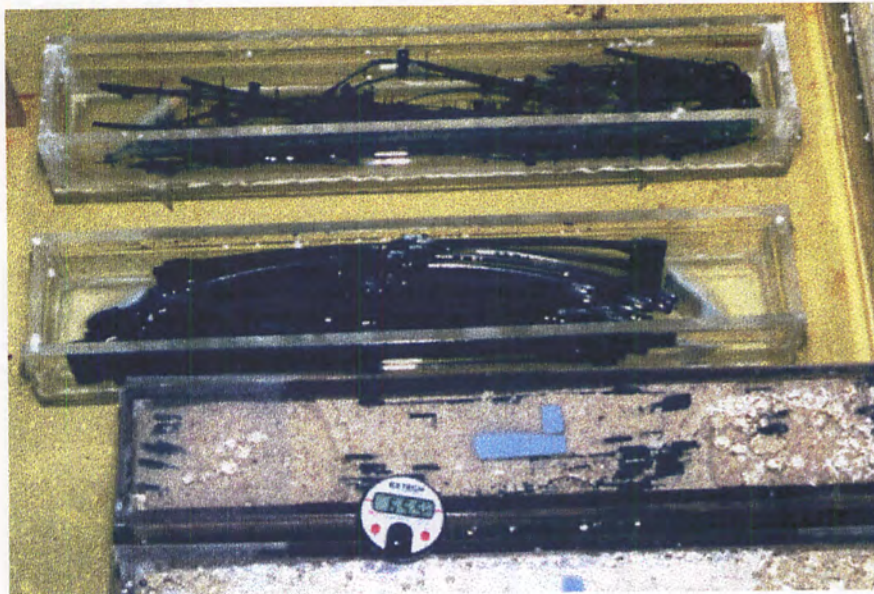
Figure 8.7 Temperature control, 65° C tank
