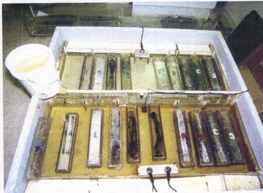
Figure 8.3 Uncovered durability tanks
