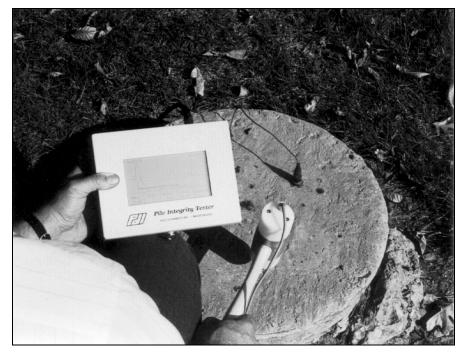
Figure 34, Pile Integrity Tester (After PDI, 1993)
