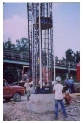
Figure 38, Osterberg Load Cells
