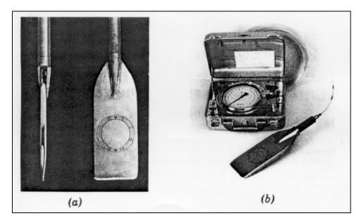
Figure 10, Dilatometer (After Marchetti 1980)
