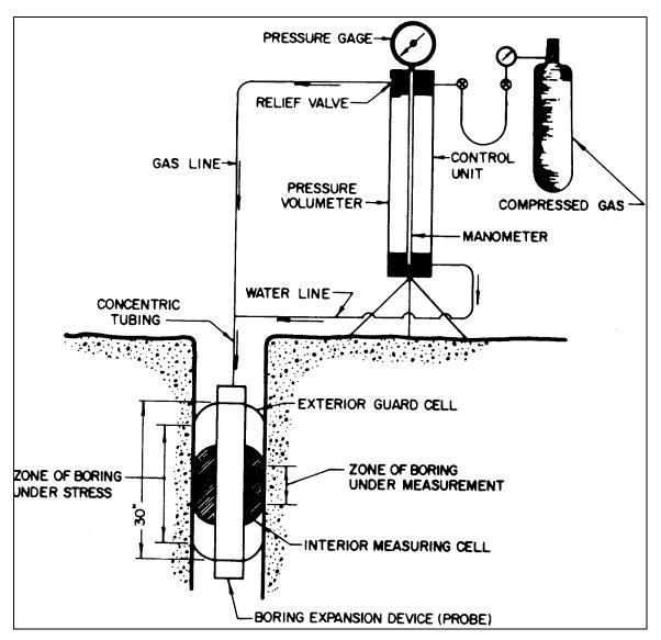
Figure 12, Menard Pressuremeter Equipment (After NAVFAC, 1986)
