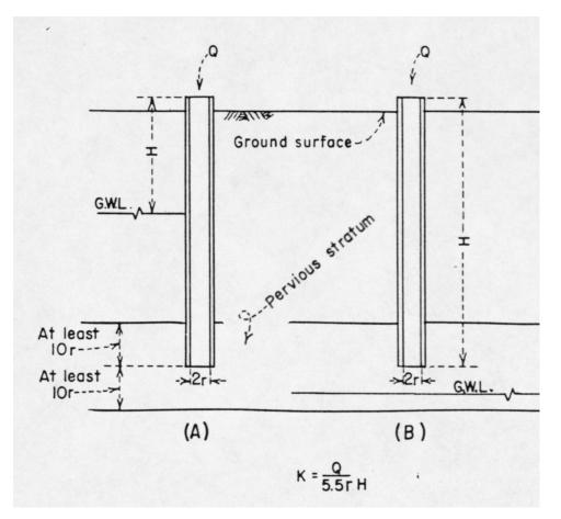
Figure 14, Open-end Borehole Test (After Bureau Reclamation, 1961)
