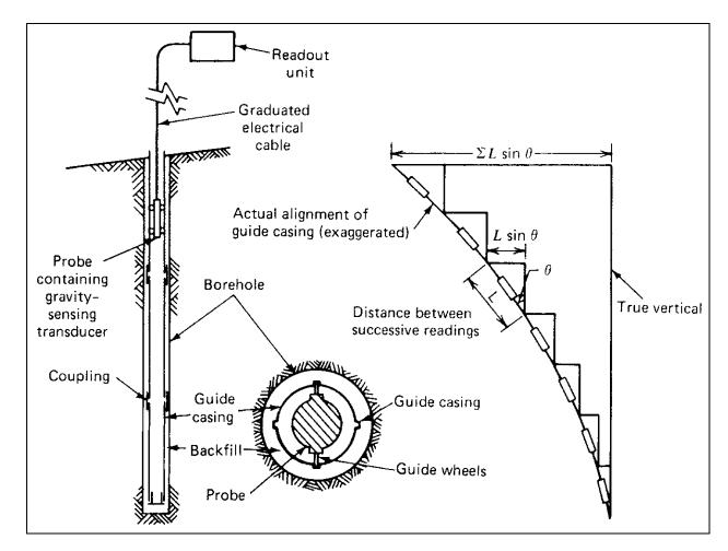
Figure 23, Principle of Inclinometer Operation (After Dunnicliff, 1988)
