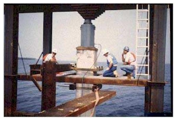
Figure 35, Static Load Test
