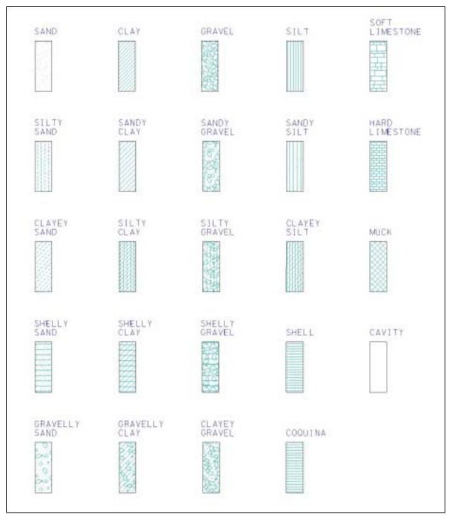
Figure 31, Standard Soil Type Symbols
