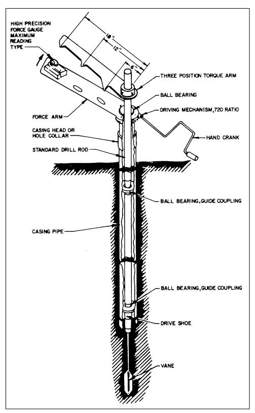
Figure 13, Vane Shear Test Equipment (After NAVFAC, 1986)
