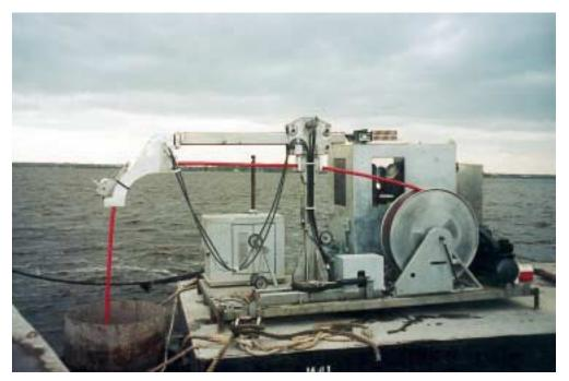
Figure 39, Shaft Inspection Device
