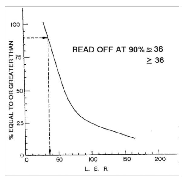
Figure 26, Design Example 1 (LBR Design Methods) 90% Method
