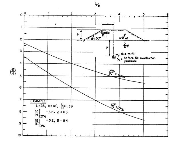
**Figure 5,** Chart for Determining the Maximum Depth of Significant Increase in Vertical Stress in the Foundation Soils Resulting from an Infinitely Long Trapezoidal Fill (both fill and foundation assumed homogeneous, isotropic and elastic). (After Schmertmann, 1967)
