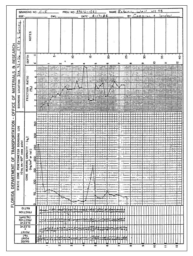
Figure 6, Typical Log from Mechanical Friction-Cone
