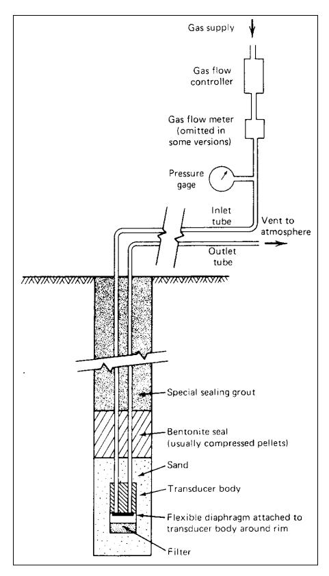
Figure 25, Typical Pneumatic Piezometer (After Dunnicliff, 1988)
