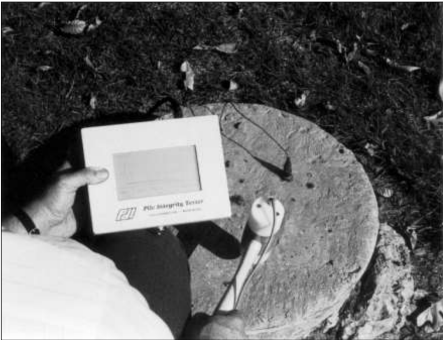
Figure 42, Pile Integrity Tester (After PDI, 1993)
