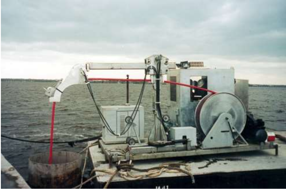
Figure 43, Shaft Inspection Device
