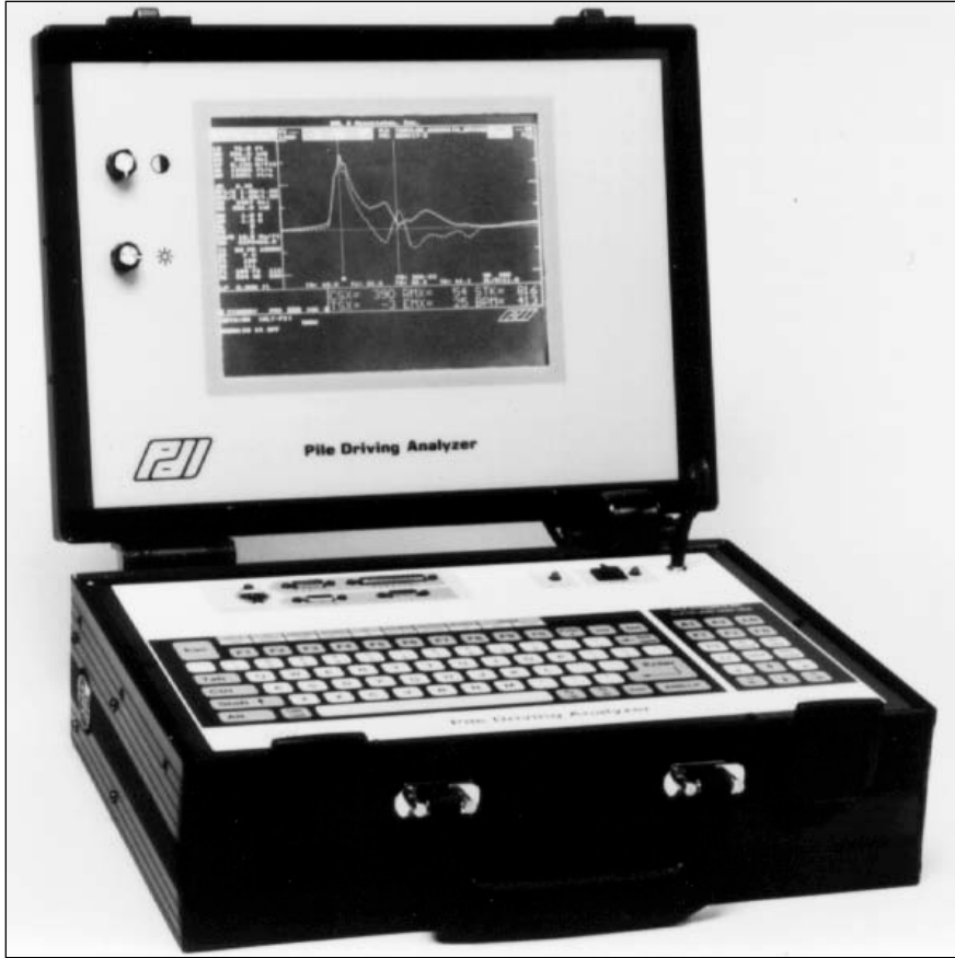
Figure 37, Pile Driving Analyzer, Model PAK (After PDI, 1993)
