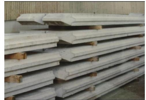
Prestressed Sheet Piles
