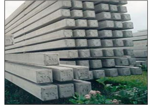
Prestressed Concrete Piles
