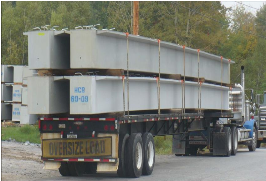
HYBRID COMPOSITE BEAMS Union St., Maine (4 - 70 ft. beams @ 9 kips = 36 kips total)
