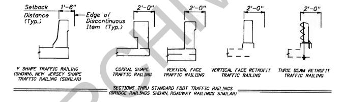
Fender access ladders are exempt from this requirement. Sign panels may be placed within the given setback distances, however the setback to the sign support may have to be increased to assure sign panels do not extend past the top inside face of the traffic railing. Motorist aid call boxes may be placed within the setback distances to allow for proper access and to meet ADA requirements, however the call box must not extend past the top inside face of the traffic railing.
