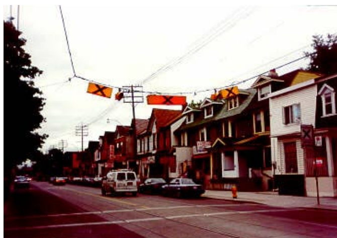
Figure 4. Toronto, Ontario, Canada has hundreds of internally-illuminated overhead signs and beacons that flash when activated.
