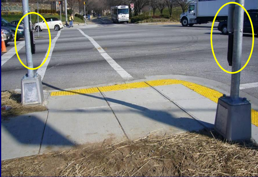
Good placement of APSs
