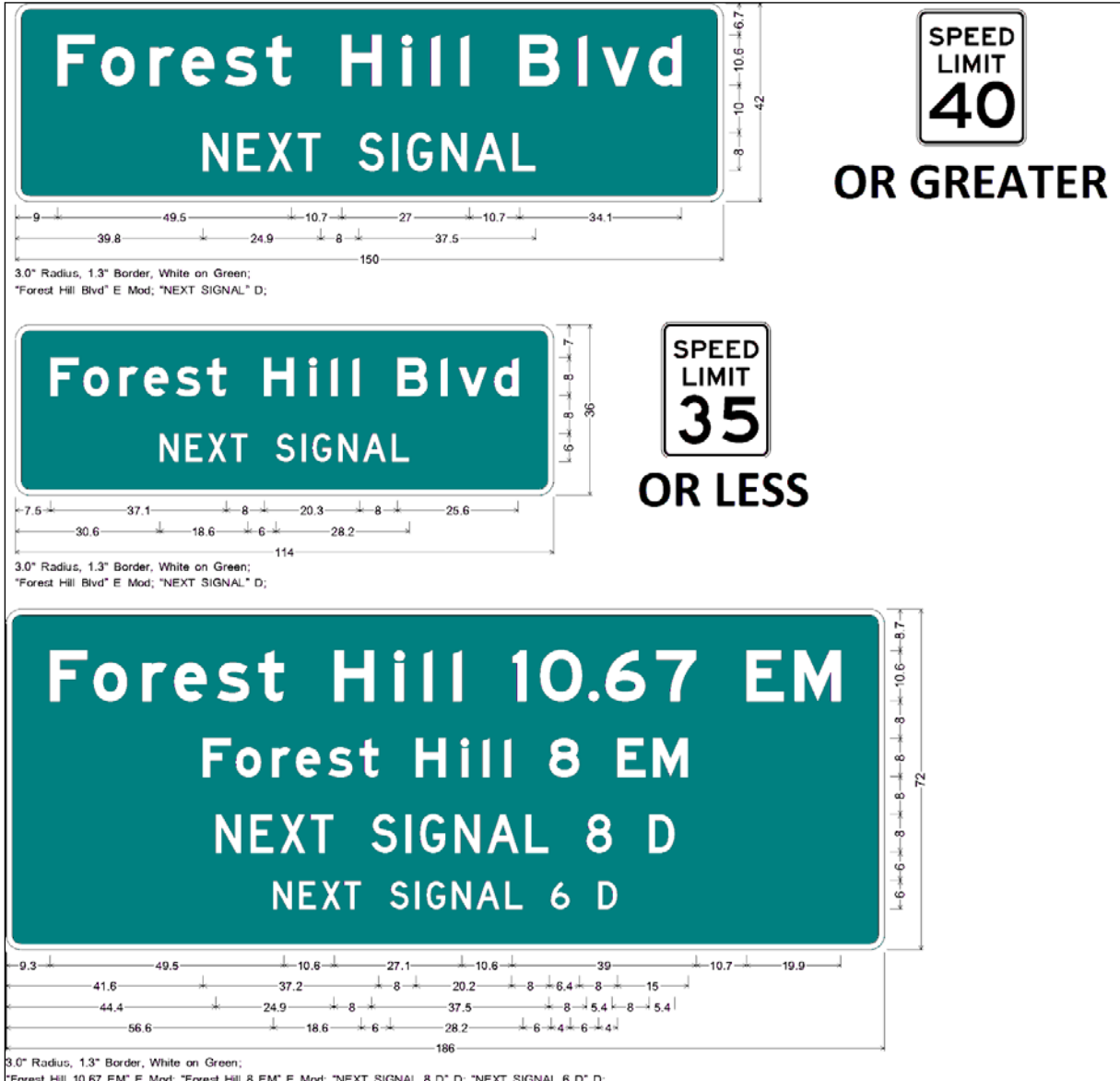
Figure 18 – 1 Examples of Advance Street Name Signs
