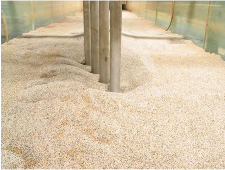
Figure 48 Post Scour Test 5 Photograph Taken From Upstream.
