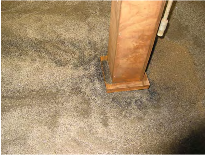
Figure 22 Post Scour Test 1 Photograph Taken From the Side.
