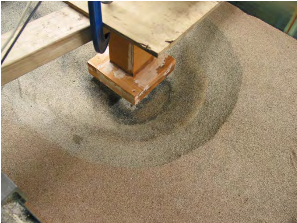
Figure 59 Post Scour Test 7 Photograph Taken From Upstream.
