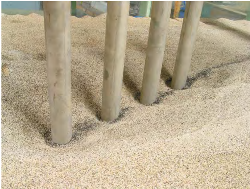
Figure 49 Post Scour Test 5 Photograph Taken From the Side of the Pier..
