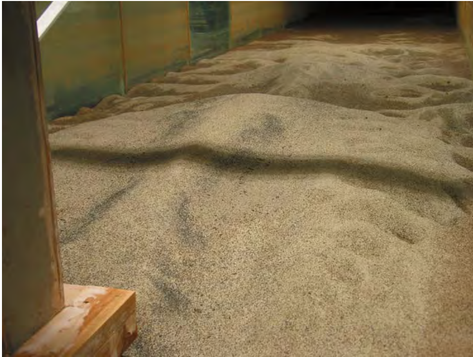
Figure 60 Post Scour Test 7 Photograph of the Downstream Bed.
