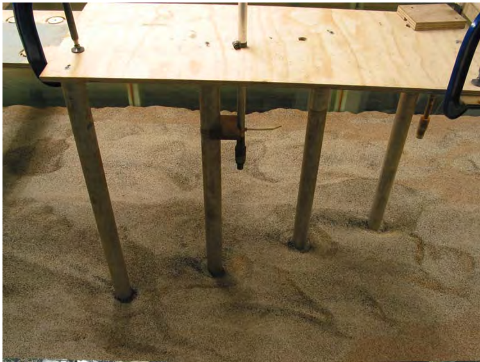
Figure 54 Post Scour Test 6 Photograph Taken From the Side of the Pier.
