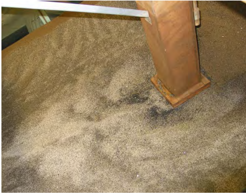
Figure 31 Post Scour Test 2 Photograph Taken From Above and Downstream.
