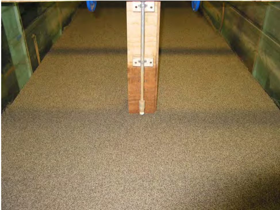
Figure 20 Pre Scour Test 1 Photograph Taken From Upstream.
