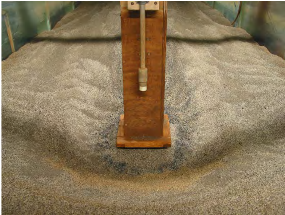
Figure 21 Post Scour Test 1 Photograph Taken From Upstream.
