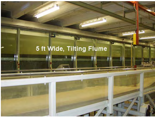
Figure 2 Side and top views of the 5 ft wide, 4 ft deep, 148 ft long flume used for the local scour tests
