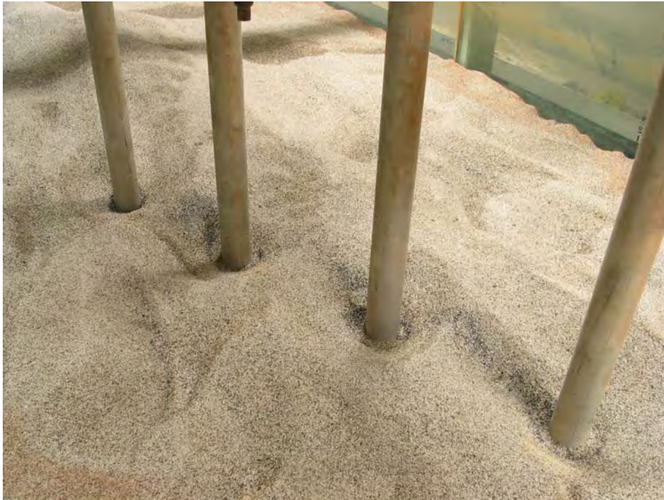
Figure 55 Post Scour Test 6 Photograph Taken From Above.
