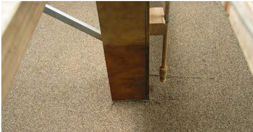
Figure 18 Side View of Pier Showing Front Face Transponder Location.
