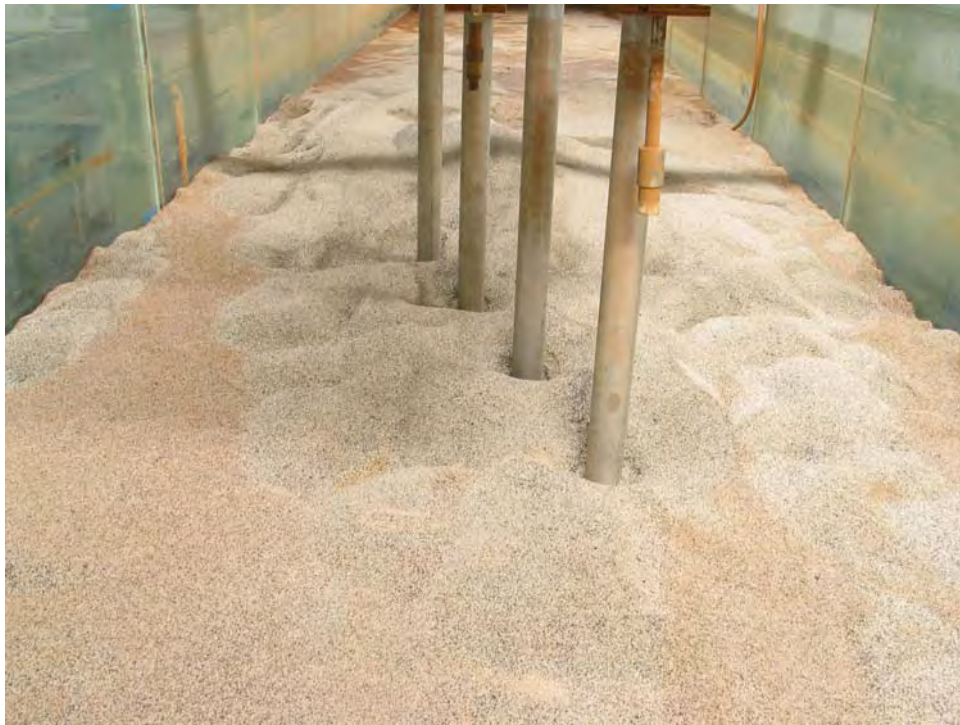
Figure 53 Post Scour Test 6 Photograph Taken From Upstream.
