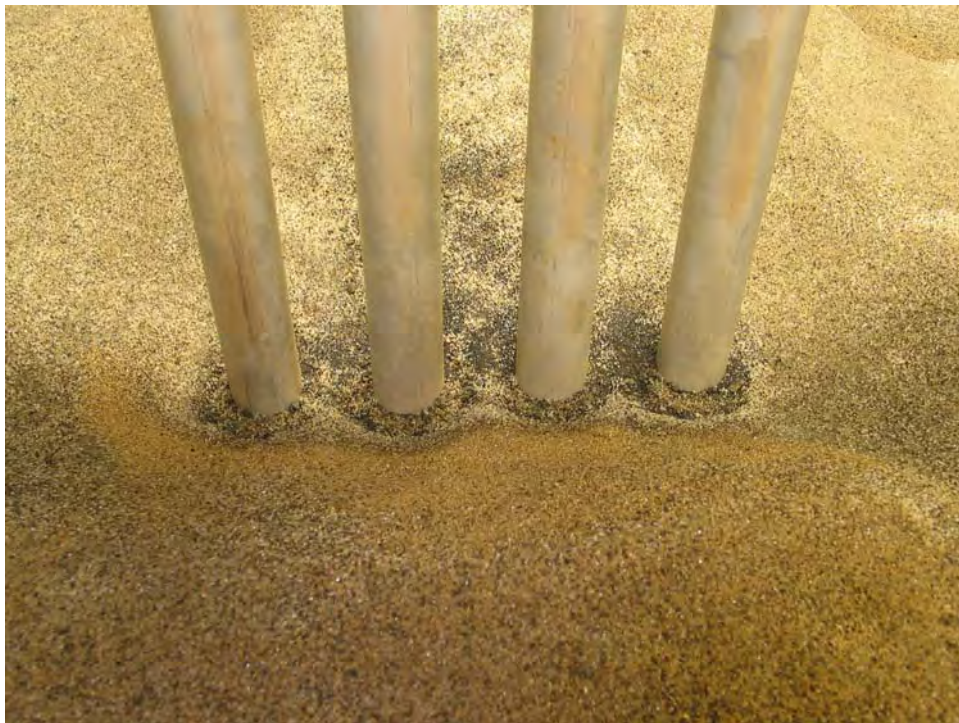
Figure 35 Post Scour Test 3 Photograph Taken From Upstream.
