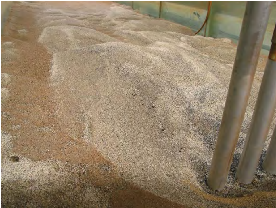
Figure 37 Post Scour Test 3 Photograph of the Downstream Bed.
