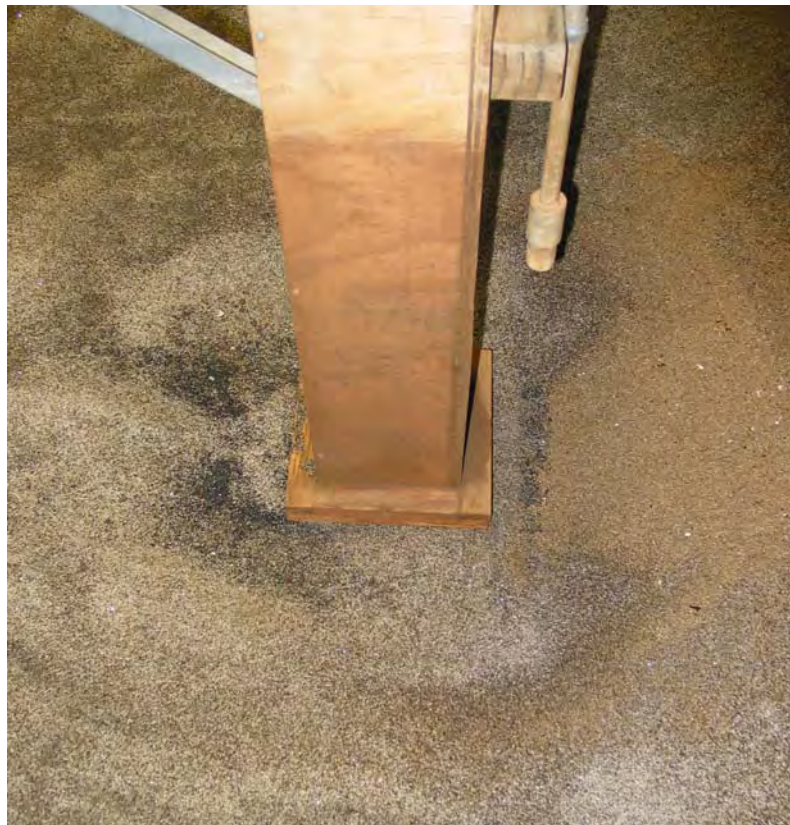
Figure 30 Post Scour Test 2 Photograph Taken From Above and the Side.
