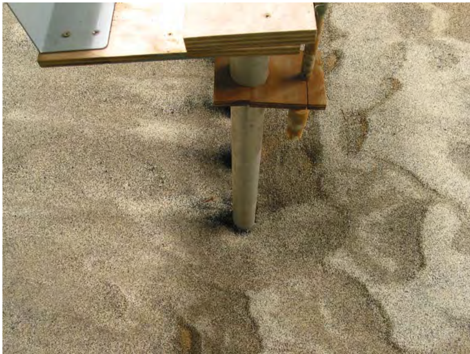
Figure 42 Post Scour Test 4 Photograph Taken From the Side of the Pier.
