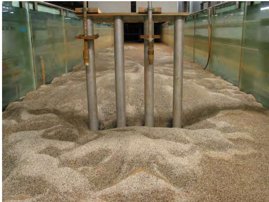
Figure 44 Post Scour Test 4 Photograph of the Overall Scour Hole Taken From Upstream.
