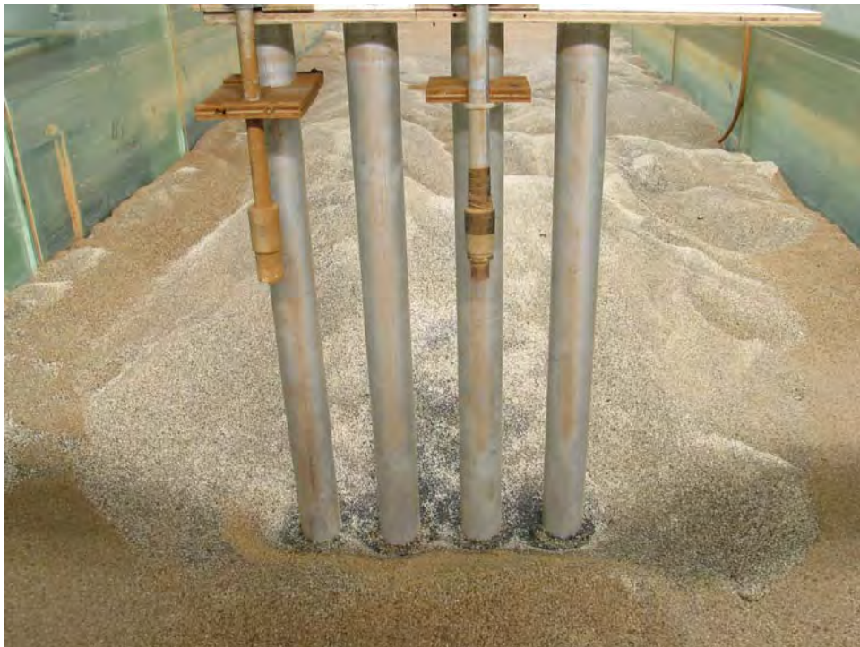
Figure 38 Post Scour Test 3 Photograph of the Overall Scour Hole.
