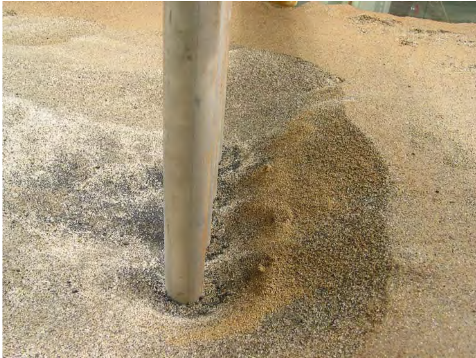
Figure 36 Post Scour Test 3 Photograph Taken From the Side of the Pier.
