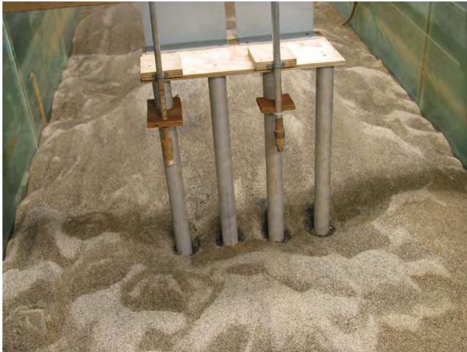
Figure 41 Post Scour Test 4 Photograph Taken From Upstream.
