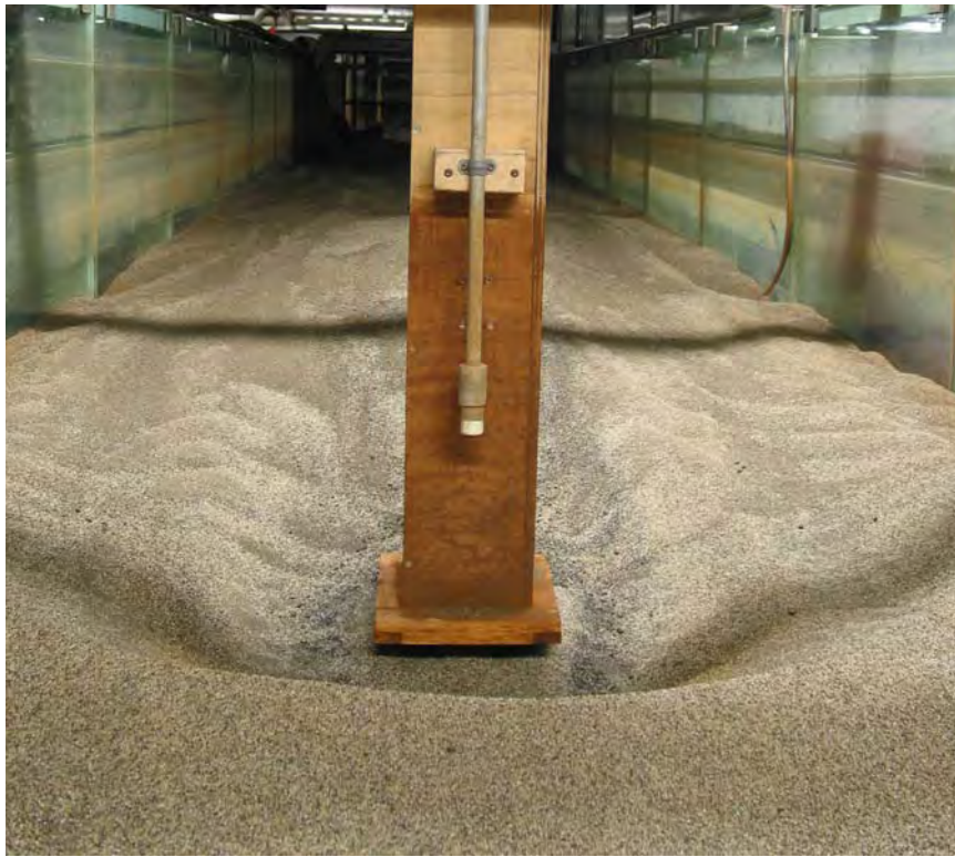
Figure 24 Post Scour Test 1 Photograph Taken From Upstream.
