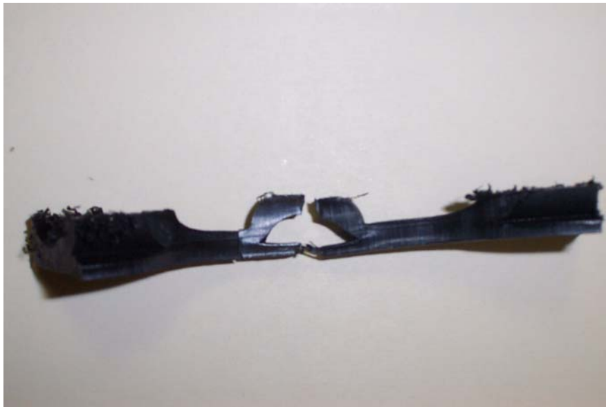
Fig. 2.9 – Failed longitudinal profile (vent hole) specimen
