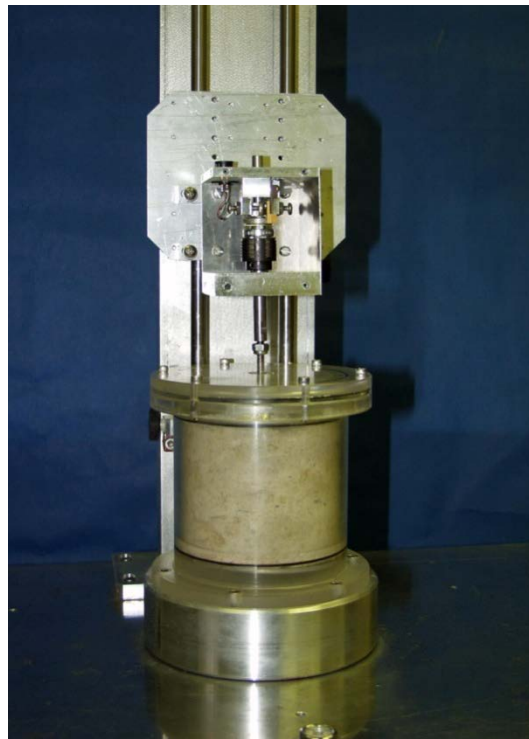
Figure 5-3 R otating E rosion T est A pparatus (RETA). The Florida Department of Transportation State Materials Laboratory currently has five operating RETAs.
