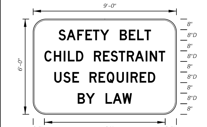
FTP-44-06 9' X 6' 9" Radii 3/4" Border 8" Series D Legend White Background Black Legend and Border
