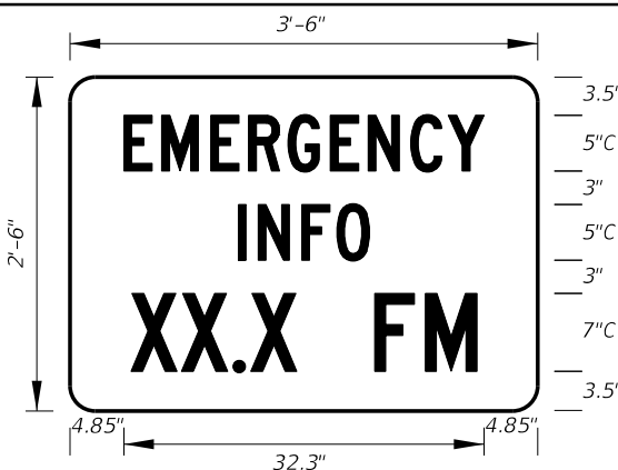
FTP-70-06 3'-6" X 2'-6" 2.25" Radii 3/4" Border 5" Series C and 7" Series C Legend Blue Background White Legend and Border
