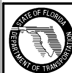
FTP-29-06 2'-0" X 1'-0" 2" Radii 5/8" Border 4" Series C Legend Yellow Background Black Legend and Border
