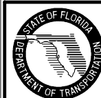
FTP-72-06 3' X 3' 2" Radii 3/4" Border 6" Series C Legend Yellow Background Black Legend and Border
