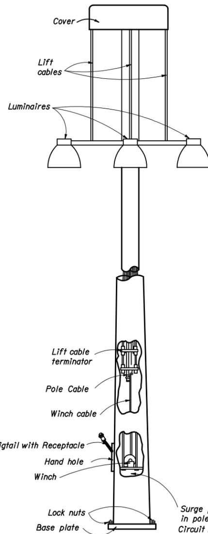
Surge protector shall be located in pole with circuit breaker. Circuit Breaker and Surge Arrester inside pole. Surge arrester to be mounted at front near hand hole for easy access.
