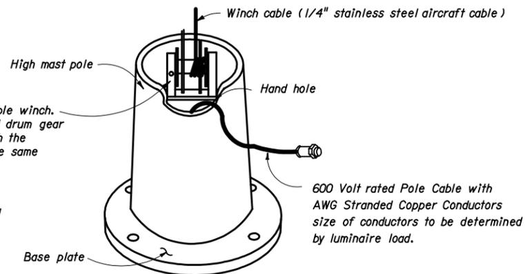
Positive drive reversible winch. The complete enclosed drum gear shall directly mesh with the worm gear train, in the same enclosure.
