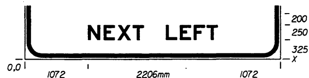
FTP - 14B 4350 X 2250 75 Radii 50 Border 250 Series E Legend White Background Black Legend & Border
