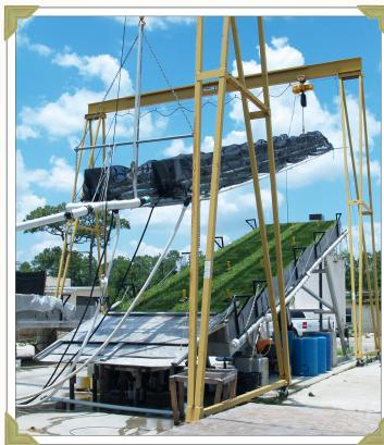
**2010:** The rainfall simulator at the Stormwater Academy at the University of Central Florida is the largest of its type in the world. The 1,500 gallon water tank can be emptied in different droplet arrangement over a bed of sod or soil set at various slopes to study runoff behavior
