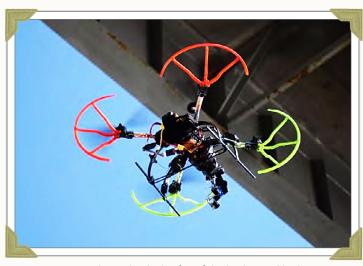
**2014:** Unmanned Aerial Vehicles (UAV) for bridge and high mast luminary inspection bring autonomous and automated technology to the maintenance work of FDOT. (BDV28 977-02)
