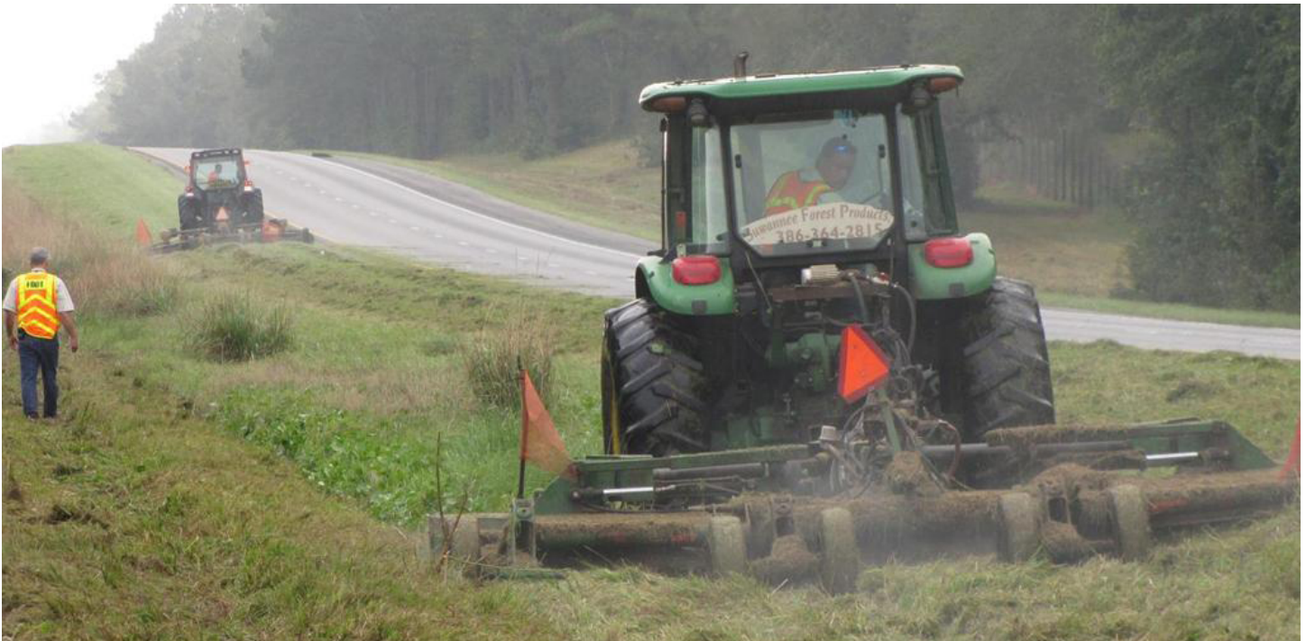
Mowing the I-10 test site in Madison County. Researchers observed no adverse impacts concerning erosion, safety, aesthetics, or turf quality at the test site. They also found that the modified mowing schedule conserved energy and saved over $1,000 per mile per year.
