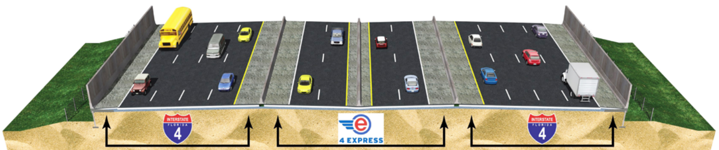
Rendering of lane configuration of the reconstructed I-4 Ultimate project. The project adds four tolled express lanes—two in each direction—to the center of the highway, while maintaining the existing free general use lanes—four in each direction. Research demonstrates that roads wider than three lanes can be sloped in one direction without compromising safe travel conditions during periods of rain.
