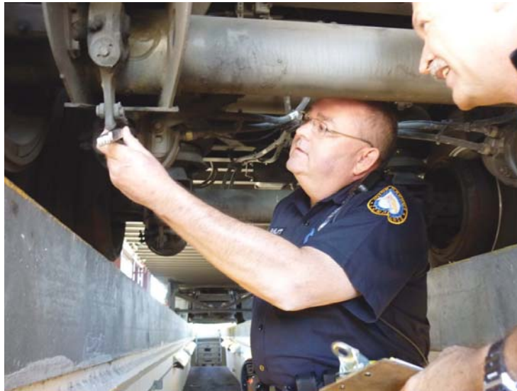
A safety inspector examines the air braking system of a commercial vehicle.
