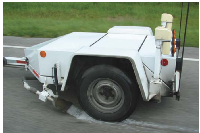
A friction trailer measures friction resistance from the force induced when the wheel is locked for three seconds over a wetted pavement surface. FDOT conducts friction tests on all newly constructed pavement surfaces, overlays, locations identified as having an unusual number of wet weather accidents, research test sections, milled surfaces, bridge decks, and other special request projects.
