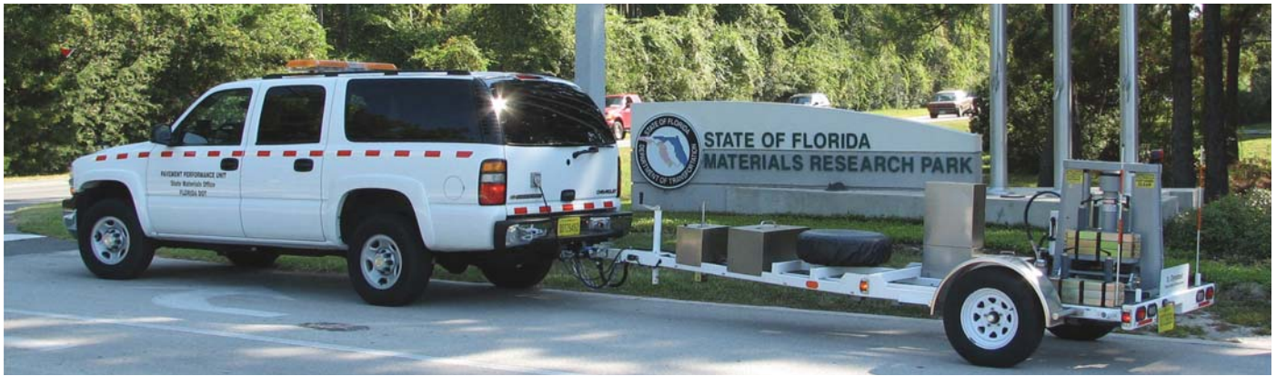
A falling weight deflectometer (FWD), shown above being towed behind an FDOT survey vehicle, is a nondestructive testing device used to evaluate the physical properties of pavement.
