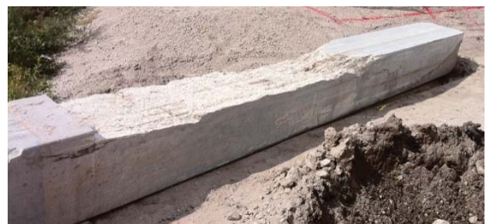
A pile damaged during driving.
