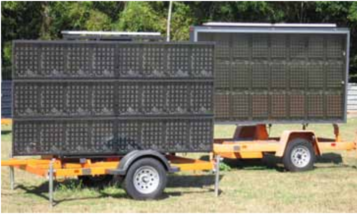
Two trailer-mounted temporary dynamic message signs (DMS) undergoing testing at TERL.
