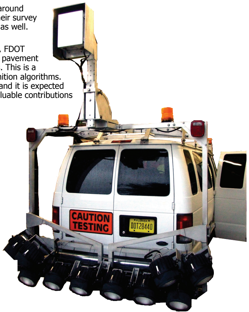
A massive light array allows data collection at night.
