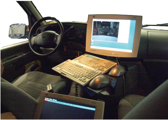
Work station for the MPSV driver.
