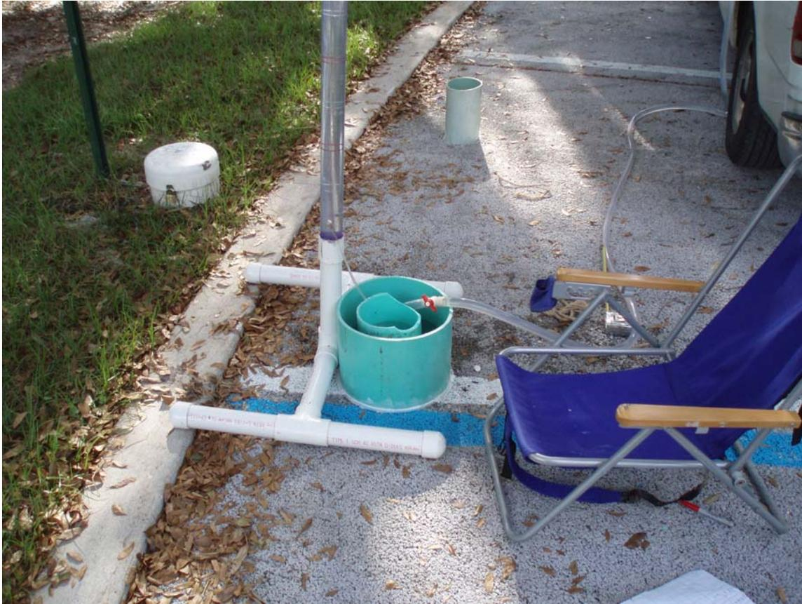
**Figure 4 - Embedded Ring Infiltrometer Kit Showing On-Site Measurement**
