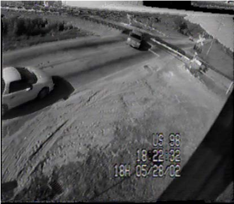
Figure 4-11: Drive-Around Violation at US 98 Site
