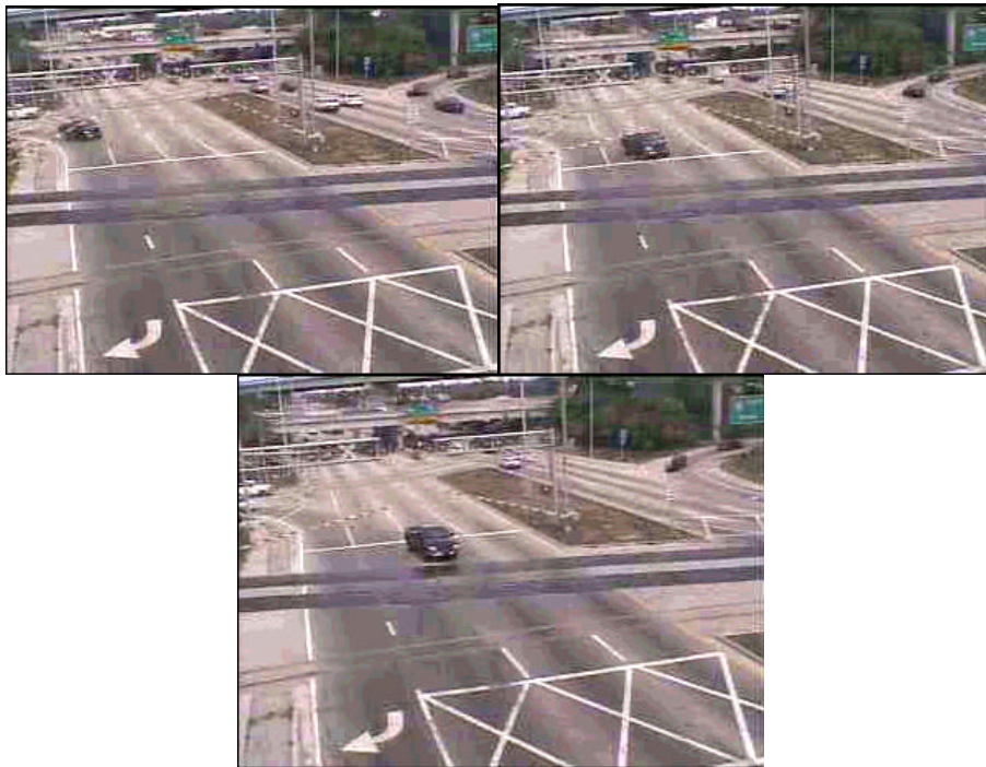
Figure 24 Vehicle Violating the Crossing Signals and Gates
