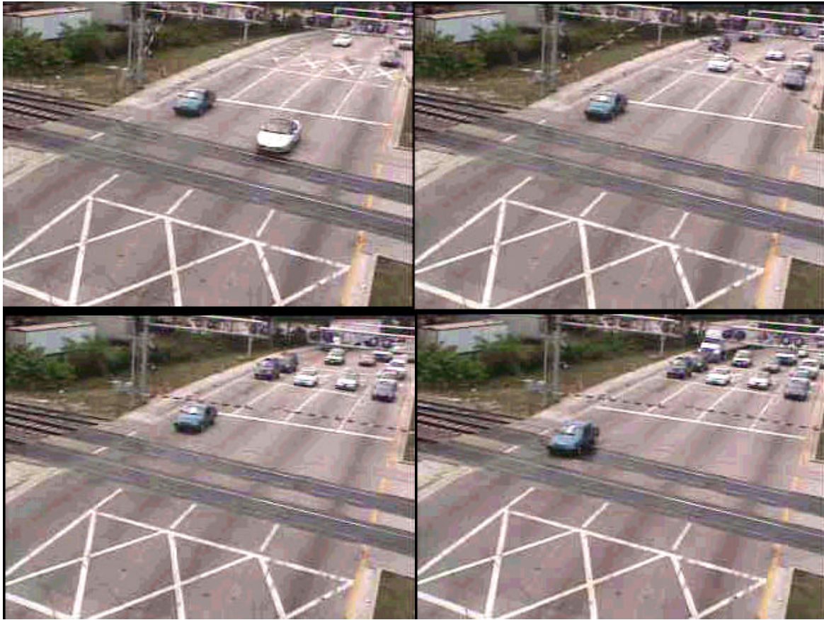
Figure 25 Vehicle Stopped in the Crossing with the Gates Down
