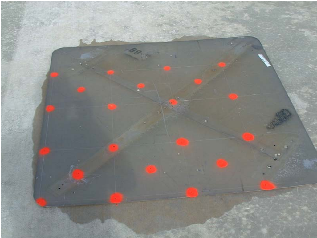
Figure 40. Steel template for marking impact and receiver locations
