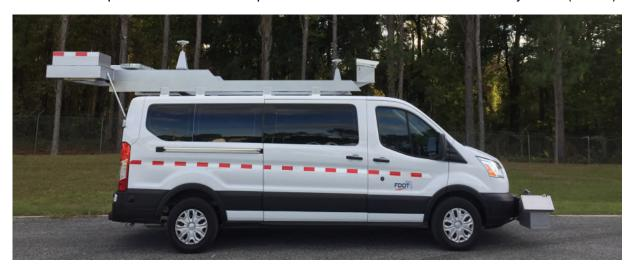
2019 – The department upgraded to using Gocator 2342 Line lasers with line at  $90^{\circ}$  (transverse) angle.
