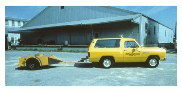
1971 -- Florida built in house a PCA Road Meter to collect data at highway speeds. Inches of displacement between the vehicle frame and axle was correlated to PSI values from the CHLOE Profilometer.
