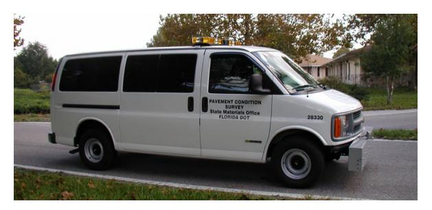
1999 -- The Department upgraded to laser sensors and started using Ride Number (RN) in addition to IRI. Ride Number is an ASTM E-1489 standard.
