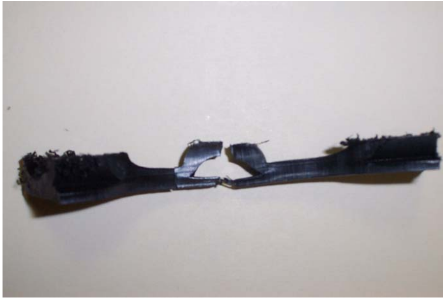
Fig. 2.9 – Failed longitudinal profile (vent hole) specimen
