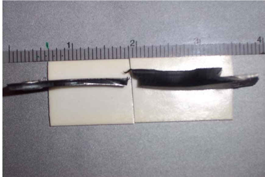
Fig. 2.7 – Failure of junction-specimen from pipe P-2
