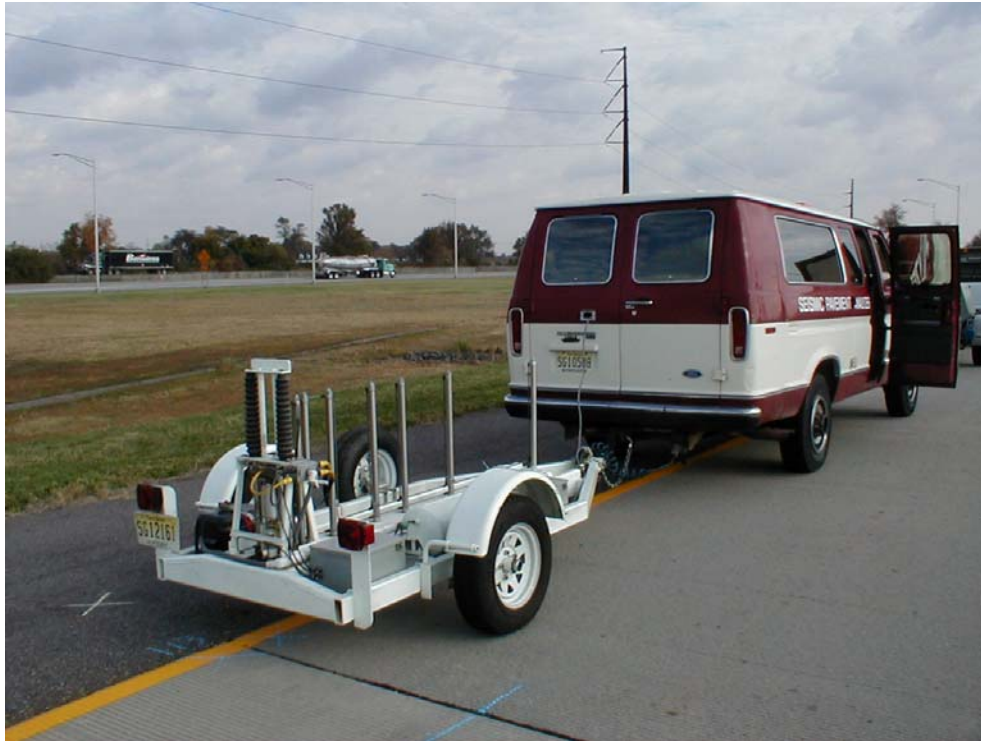
Figure 2- SPA testing on a rigid test section.
