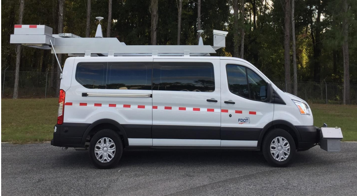
FIGURE 1. LCMS w/ INERTIAL PROFILER
